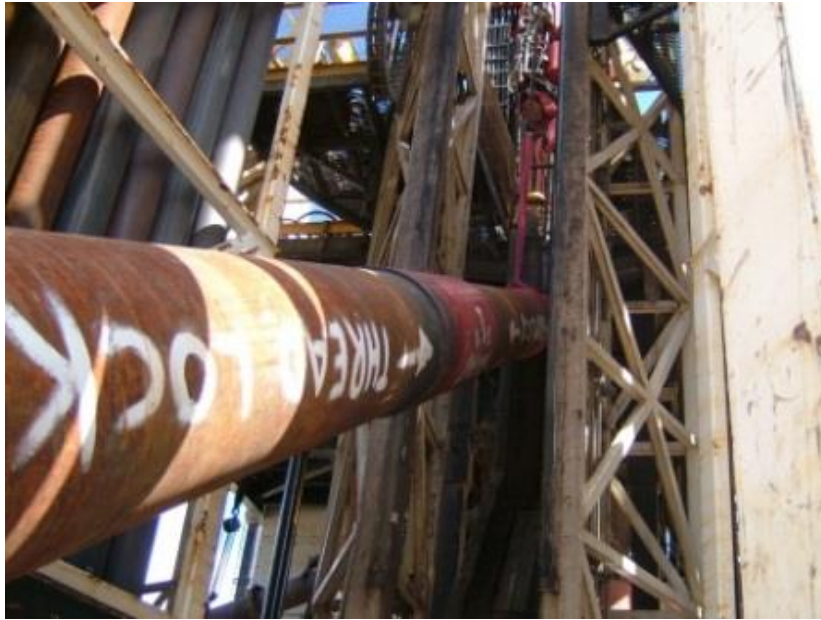
Lower and attach Elevator to casing
