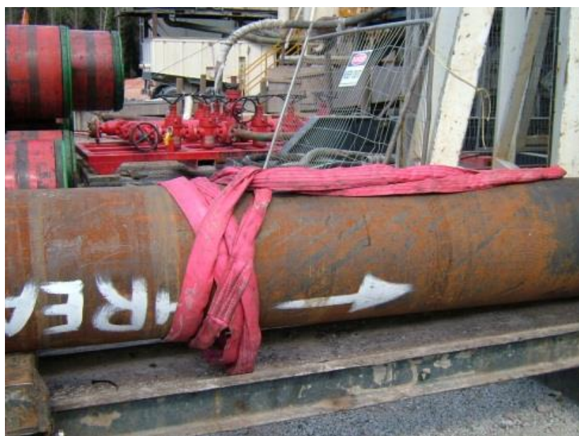
Soft sling attached to casing
