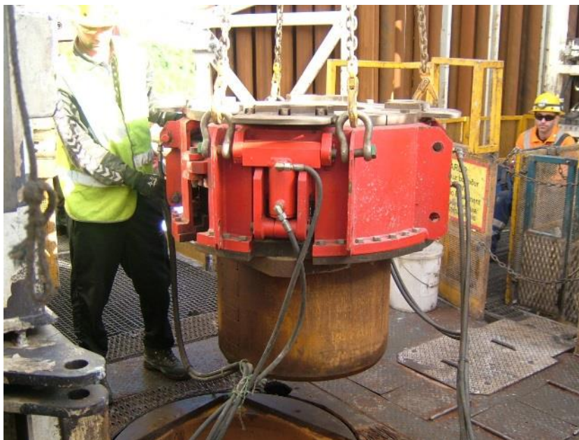
Casing slips in place.
