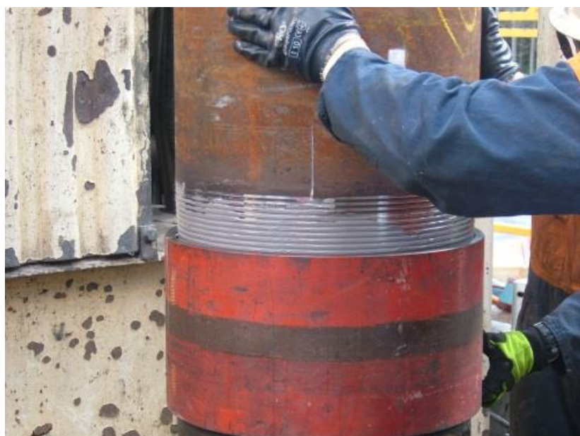
Rotate casing and make up using top drive make-up
