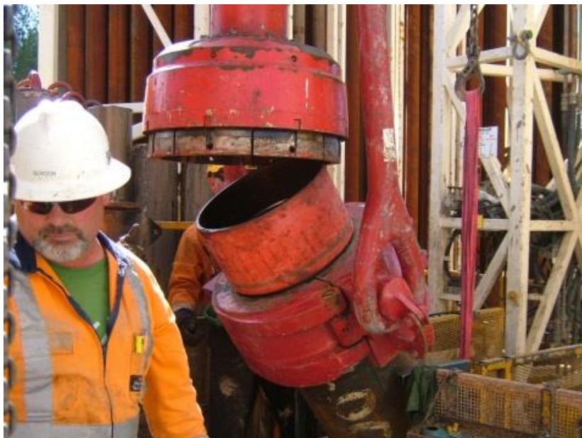
Ensure casing collar comes inside casing make up device
