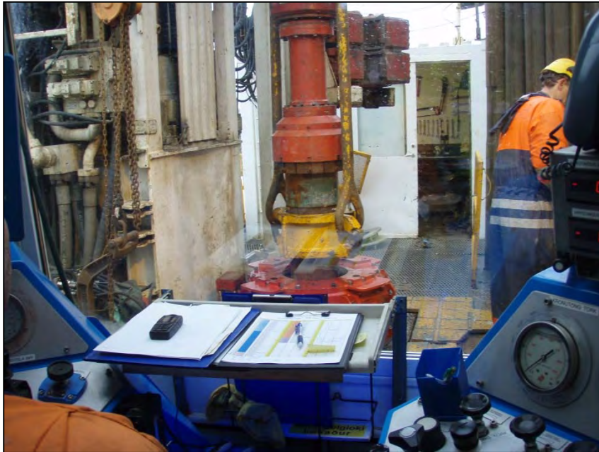
Casing lowered into casing slips
